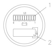
Every column means 10% Two electric bars show on battery charge used up warning. The battery must be charged.
